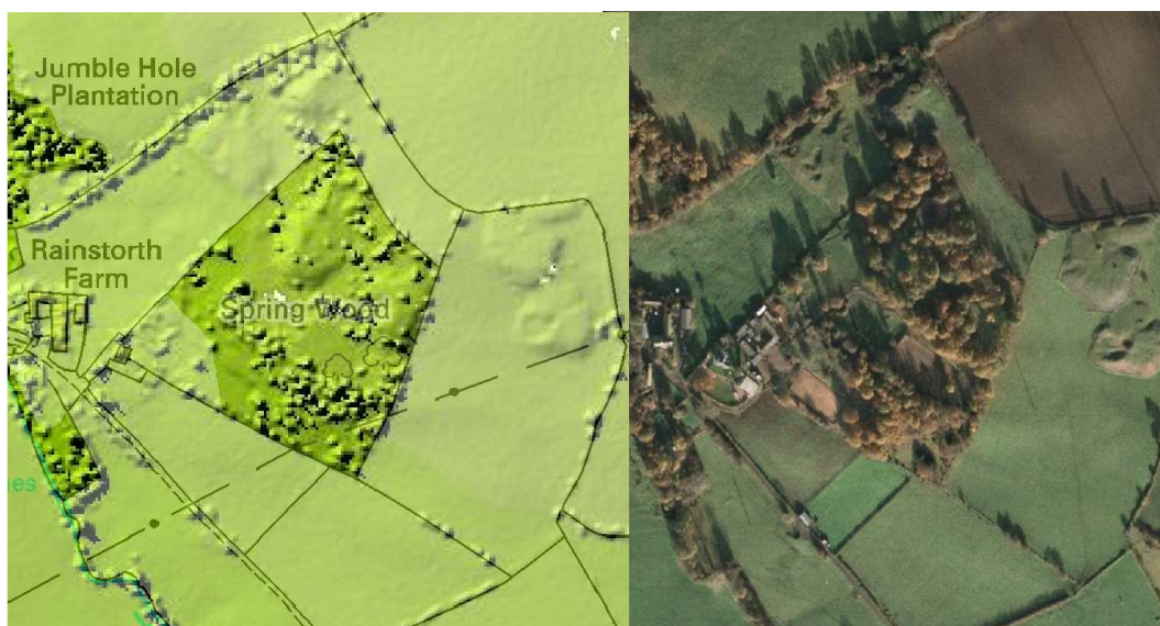
Figure 2: LIDAR survey has the potential to reveal earthworks (such as these probable annular spoil heaps within Spring Wood) that are poorly visible on vertical aerial photographs.
